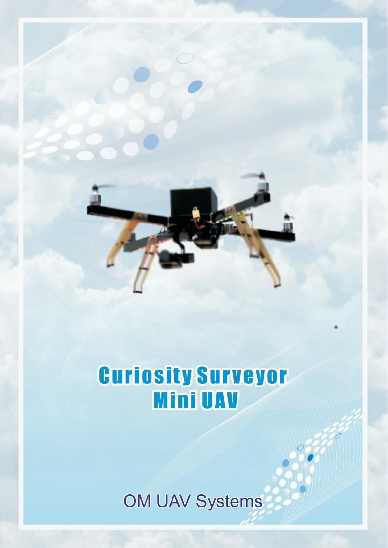
Curiosity is a FULLY AUTONOMOUS Mini Unmanned Multicopter aircraft. It is capable of carrying a 400 Gram payload. The payload is a Day or Night Camera mounted on a gyro stabilized camera mount. Most cameras are under 300 Grams. The UAV is electrically powered with a very low dB level. The aircraft is fully autonomous right from Takeoff to Landing. The UAV is made of composite sheet and aluminum alloy.
